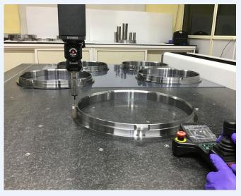
casing rings > 600 mm diameter getting inspected at SAP Parts
